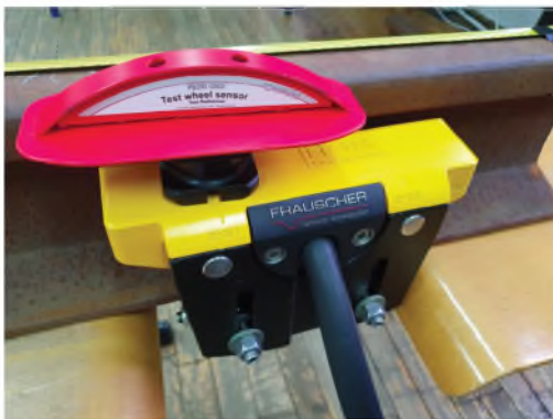
Czujnik koła | Axle counter
