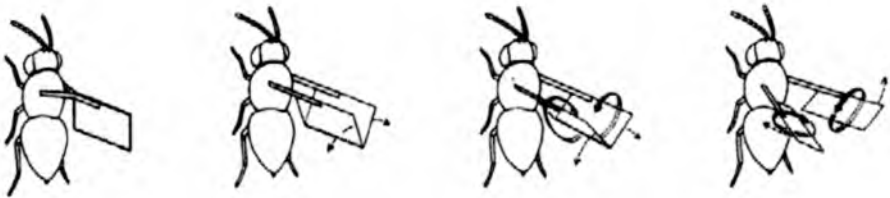
Fig. 5. Weis-Fogh clap and fling mechanism illustrated on an Encarsia Formosa . From Weis-Fogh [25]
