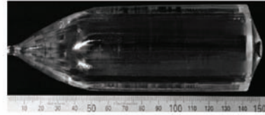
Fig. 18. 2 inch size \{Tb_3\}Sc_{2-x}Lu_x\}(Al_3)O_{12} single crystal grown by the Czochralski technique, presented by Fujikura Ltd.
