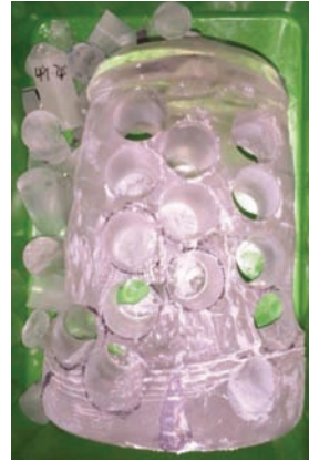
Fig. 2. A Kyropoulos-grown sapphire crystal after core drilling 2" rods and ready to be recycled into the growth process along with several broken or rejected rods.
