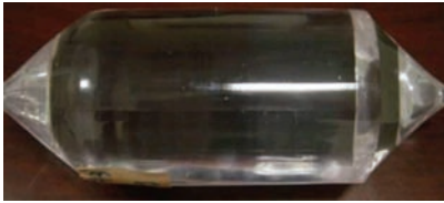
Fig. 8. A 4" c -axis sapphire crystal grown successfully without LAGBs. Note the smoother exterior surface.
