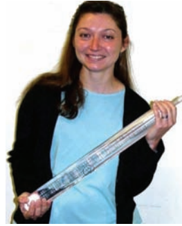
Fig. 4. One of the authors holding a 2” diameter, 18” long c -axis sapphire crystal grown free of LAGBs.
