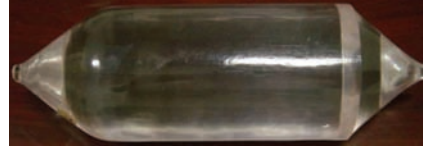
Fig. 5. A 4” diameter c -axis sapphire crystal grown at Sino-American Silicon. The surface texture is an indication of lineage.
