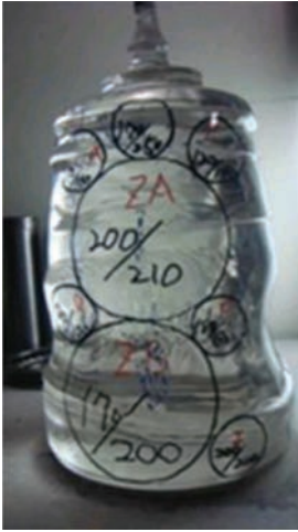
Fig. 1. A 90 kg Kyropoulos-grown sapphire crystal mapped for core drilling two 6" rods and several 2" rods.
