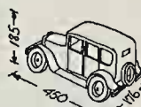
5 PERS. BIL 6-7 PERS. L: 475. BR: 180 LIMOUSINE: L: 515. BR: 185. H: 190 BABYCAR: L: 300-330. BR: 128 H: 162.
