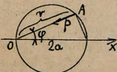
$$r^2 \frac{d\varphi}{dt} = \text{stać } C, \frac{d\varphi}{dt} = \frac{C}{r^2}. \text{ Całko-} \\ \text{wite przyjb. } p = P_r = \frac{dr}{dt} - \\ - r \left| \frac{d\varphi}{dt} \right|^2 = \frac{dr}{dt} - \frac{C^2}{r^2}.$$
