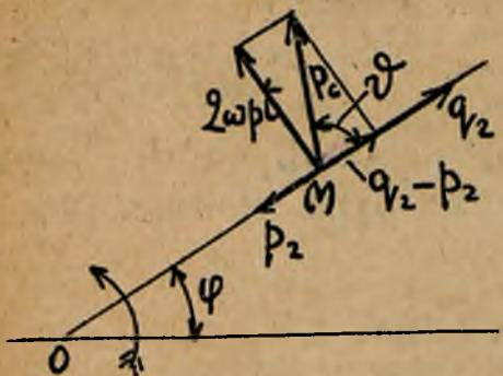
$$\operatorname{tg} \vartheta = \frac{2\omega pt}{b - p^2 t^2 \omega^2} = \frac{4wt}{2 - t^2 \omega^2};$$
