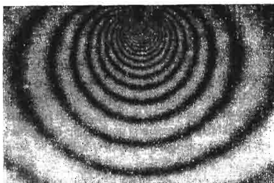
Fig. 2. Isopachic fringes of dynamic crack propagation in PMMA three-point bend specimen at crack velocity of 400 m/s
