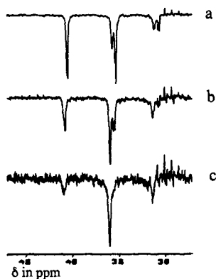
Fig.4. ^{13}\text{C} -NMR spectra of novolak resins: a - conventional b - hyperbranched novolak (first generation) c - hyperbranched novolak (second generation)
