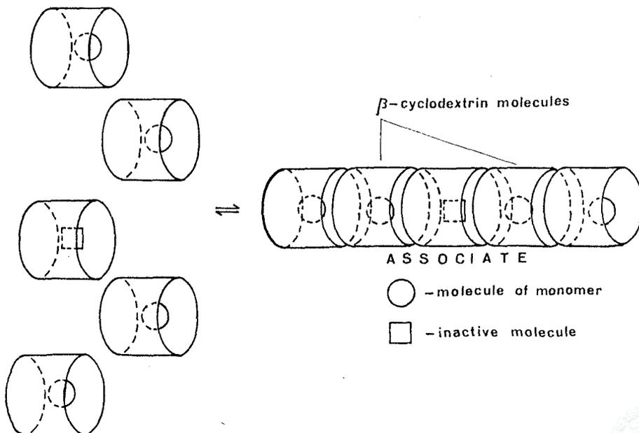
FIG. 2. Schematic diagram of the polymerization process.
