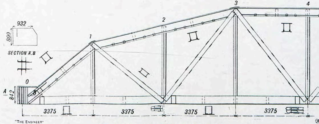
Fig. 2—Main Girder of Arc-Welded Bridge
