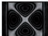
Enhanced time average fringes of vibrating membrane
