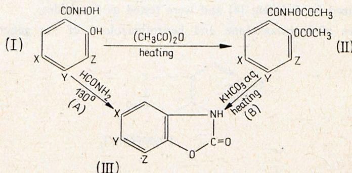
Therefore it appeared that the diacetyl derivatives of halogensalicylhydroxamic acids undergo Lossen rearrangement with simultaneous hydrolysis of the acetyl group attached to the phenolic hydroxyl, which enables the cyclization reaction to the benzoxazolone.
