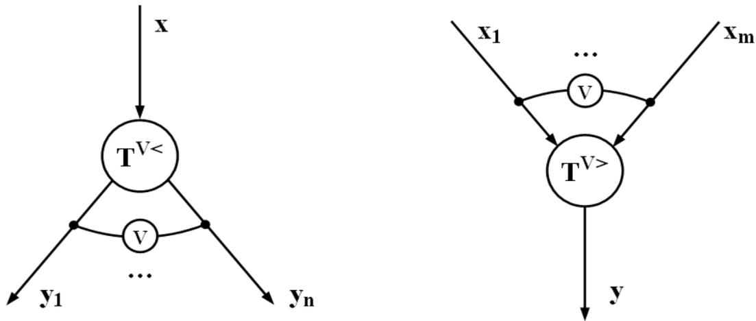
Figure 1c. T-net alternative transformers (*source: self study*)
