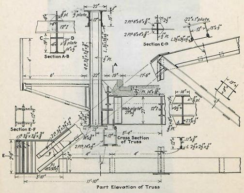
FIG. 5-STRUCTURAL DETAILS OF WELDED HIGHWAY BRIDGE IN POLAND
